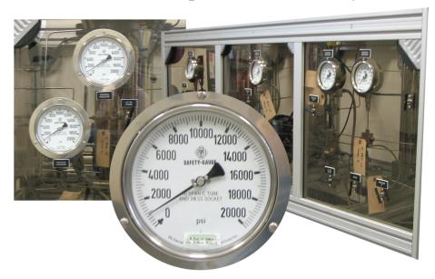
The expanded qualification of non-metallic sealing material capabilities includes NORSOK M710 Rev 2 (Annex A and Annex C) aging in high temperature/high pressure environments in fluid to measure the change in mechanical performance and chemical degradation.
